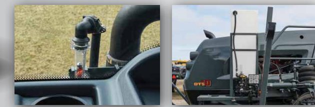
Injection unit shown installed on DTS10.
