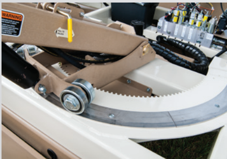
Turntable features 3/4" increments
