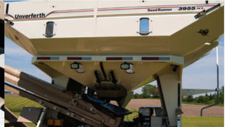
Windows and lights for fill level
