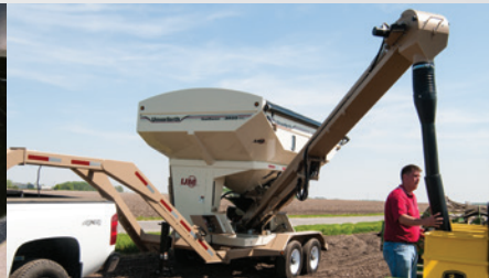
2-stage telescoping downspout
