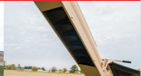
Access panel with tool-free removal
