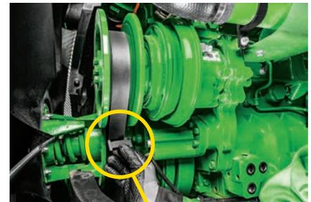
Checking Vari-Cool Fan drive belt width for wear is a very important routine maintenance step to avoid downtime. Use belt gauge R569237 shown in the picture above, which can also be purchased at your local John Deere dealer.
